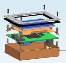
This human interface device is based on an ARM7 processor running at 72MHz. With a small form factor of 3.6" x 2.7" and wide supply voltage range, it can be utilized in several different applications. Additional flexibility is achieved with the support of several RGB and LVDS LCD panels with sizes that range from 3.5" to 10.4" and with a resolution up to 1024 x 768, which makes this HMI extremely adaptable to a wide range of applications.
